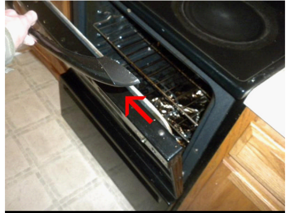
Oven door handle is broken
